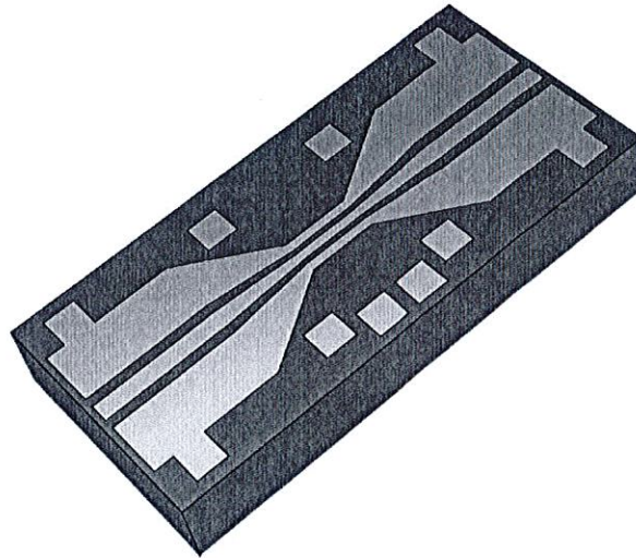
Figure 2: The integrated CPW with the Py/Cu/Nb stack underneath the central line used for the FMR measurements.
